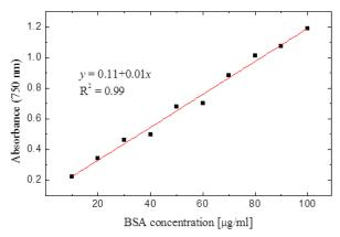
Figure . Protein standard curve performed using bovine serum albumin (BSA) as standard. The straight line represents a linear fit of measured data
